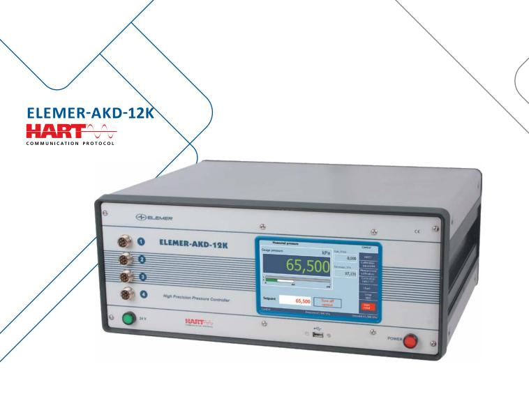
ELEMER-AKD-12K Pressure Controller reproduce and measure reference pressures. ELEMER-AKD-12K can also measure standard pressure transducer signals, check DM relay status, calculate errors, and generate verification reports
